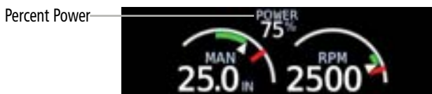
Percent Power Indicator
