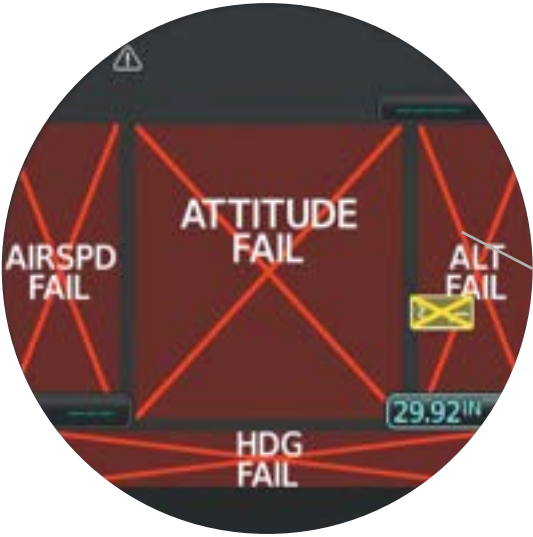
Example of Failure Annunciations
