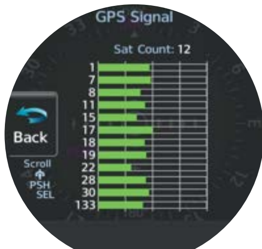
VFR GPS Satellite Signals
