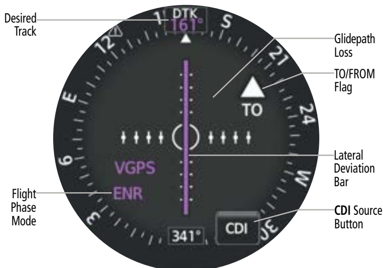
Typical 'CDI' Page with External GPS Navigator
