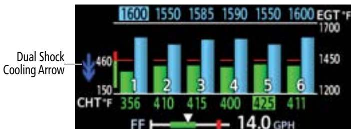
CHT/EGT - Shock Cooling - Double Arrow
