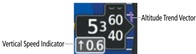
Vertical Speed Indicator and Altitude Trend Vector
