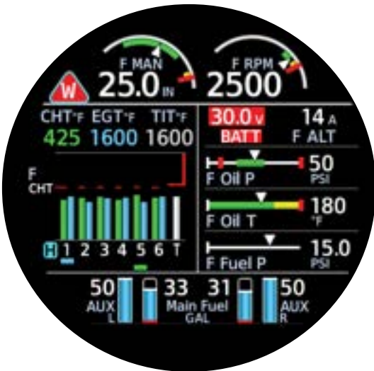
EIS Alerts - Warning - Battery Voltage
