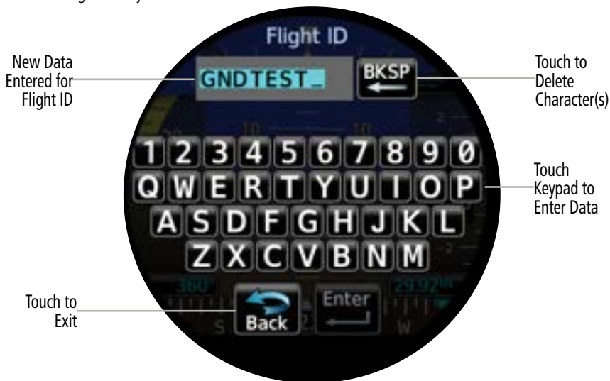
Flight ID Keypad Entry
