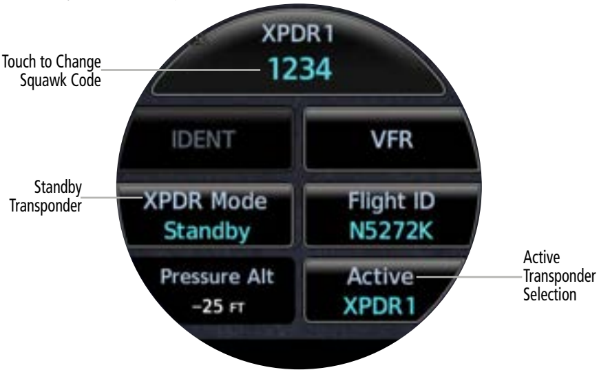
ADI - Transponder Control Display - Change Squawk Code
