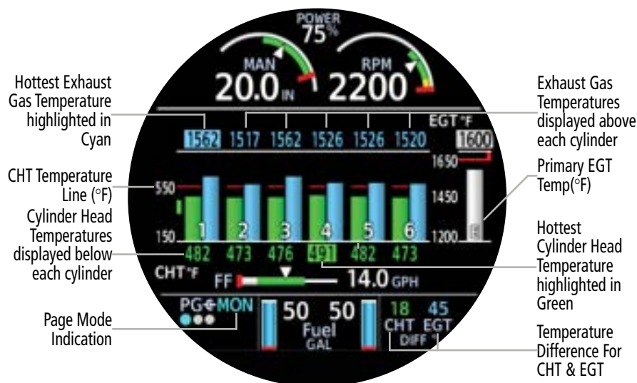
CHT/EGT - Six Cylinders - Primary EGT Temp
