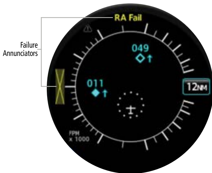
RA Failure Annunciations
