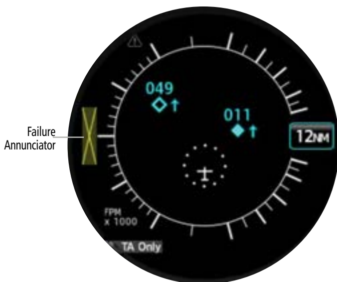
Vertical Speed Failure Annunciations
