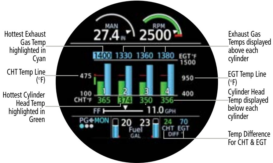
CHT/EGT - Four Cylinders - Bar Graph Example
