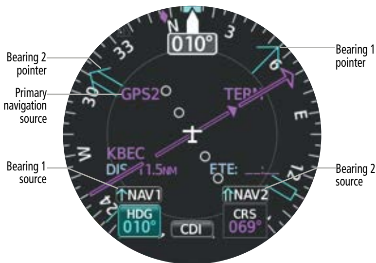
'HSI' Page with Bearing Pointers
