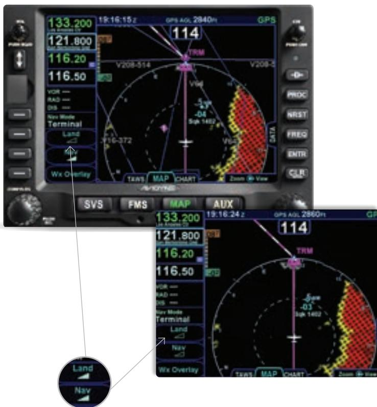
**To select the preferred level of map density displayed**, from the Map Page, Map tab, press the “Land” LSK to declutter the terrain base map and/or “Nav” LSK to declutter off-route NavAids (Intersections, Airports, VORs etc). There are four levels of declutter for each. The specified level of detail will remain consistent across all map pages. (Terrain Awareness alerts and nearby Traffic are not affected by declutter settings.)
