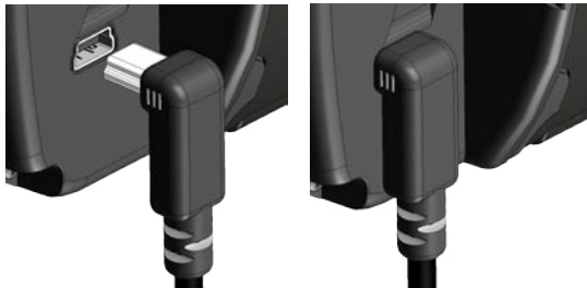
GXM 30 Antenna Plugged In
