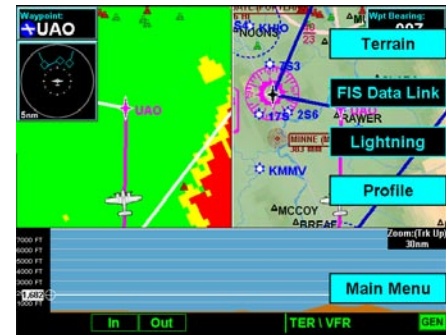
Split Screen showing Custom Map and Flight Plan pages along with the Vertical Profile & Menu Items
