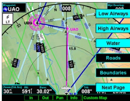
Custom Map page with Low Airways, High Airways, and Menu Items (Page 3)
