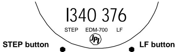
The term **tap** will be used to denote pressing a button momentarily. The term **hold** will be used to denote pressing and holding a button for five seconds or longer.
